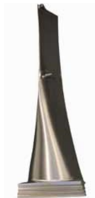
15: Steam turbines blade made of steel and titanium alloy
