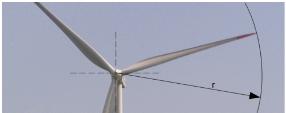
11: The rotor of the Vestas V90 wind turbine with a column height of 105 m, a rotor diameter of 90 m and an installed capacity of 2 MW. Drahaný (CZ).
