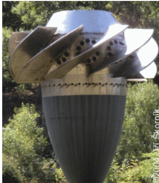
1: Kaplan turbine – rotor
