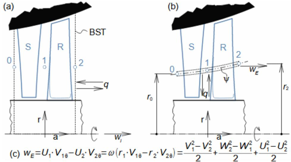
4: Difference between Euler work and internal work of stage
