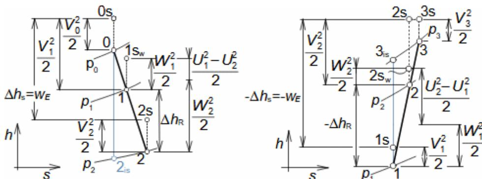
6: *h-s* diagrams of turbomachine stages
