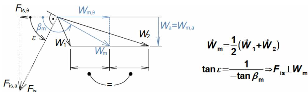
3: Definition of the mean aerodynamic velocity in the blade row and its relation to the force vector acting on the elementary blade (blade length  $dr$ )
