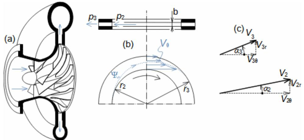
(a) rotor-bladeless diffuser assembly and inlet and outlet casing; (b) bladeless diffuser section; (c) absolute velocity at the inlet and outlet of the bladeless diffuser.
