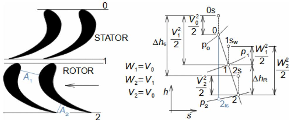
7: Example of turbine axial stage blade passages with reaction of 0,5
